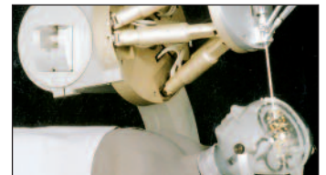
Custom Hexapod designed for neurosurgery Photo: IPA
